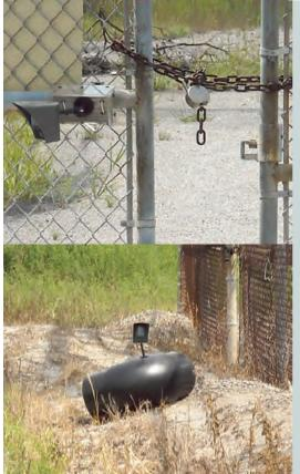
This MotionViewer was mounted directly on the front gate. Because they are "unplugged" and require no AC power, they can be installed where they are most effective.
